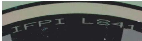
Image no. 12 – IFPI code on an optical medium (CD DVD)
